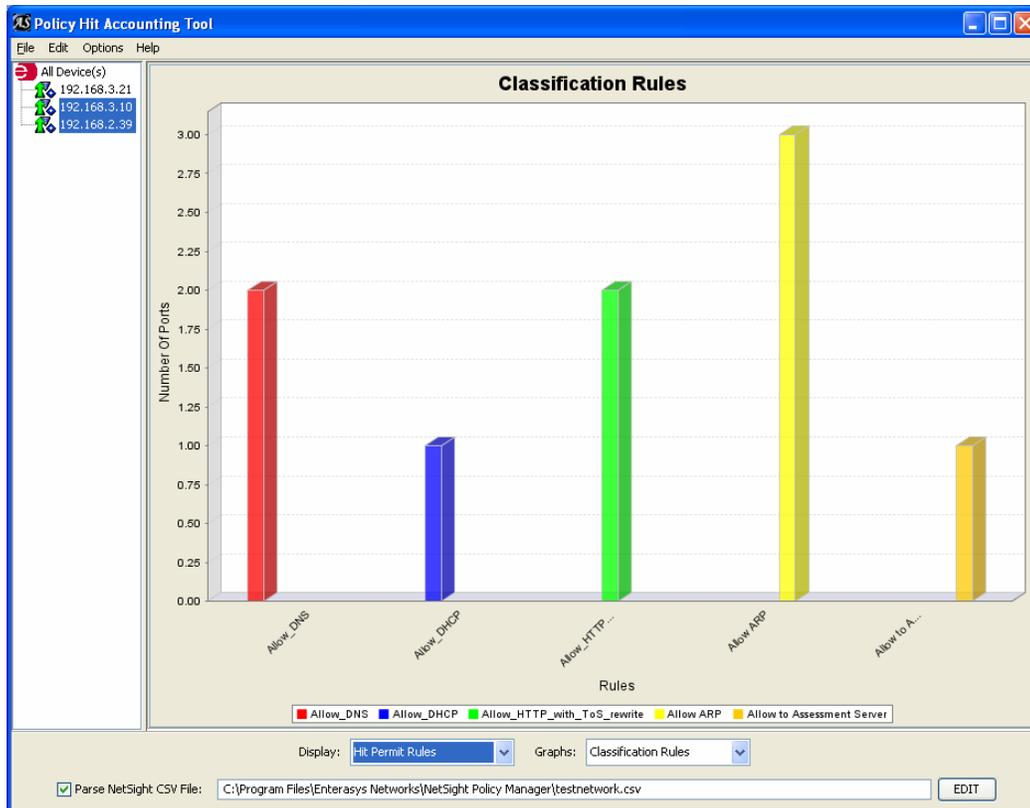
**Figure 7. Displaying classification rule names by importing NetSight Policy Manager configuration**
